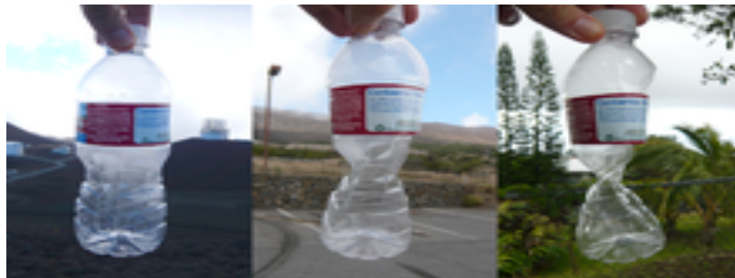
The bottle above was sealed at 14,000 feet on the left. In the middle picture, the bottle was crushed by atmospheric pressure at 9,000 feet. The picture on the right shows the effect of atmospheric pressure at sea level.
